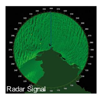
The marine renewable industry, and anyone who uses coastal waters, need a detailed understanding of waves and currents. X-band radar can transform our capability for measuring these, broadening our view from a single point to a whole section of sea. The WDNA has accelerated our efforts to develop this exciting new technology here in Wales.
